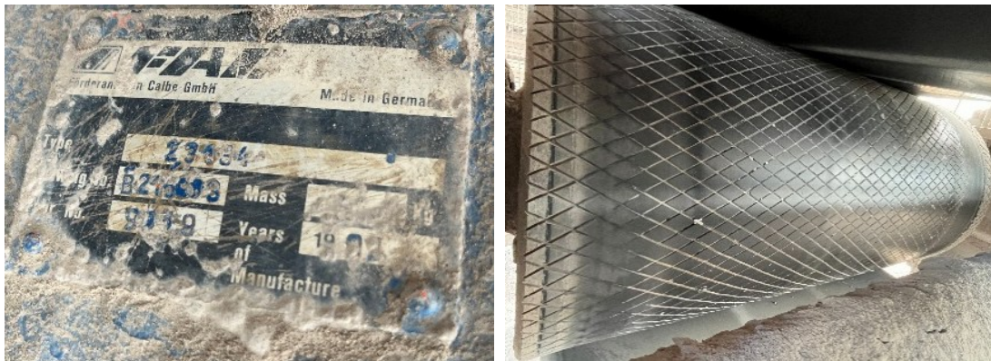
Figure 3: Conveyor tail pulley item no. 2 in Table no. 1
